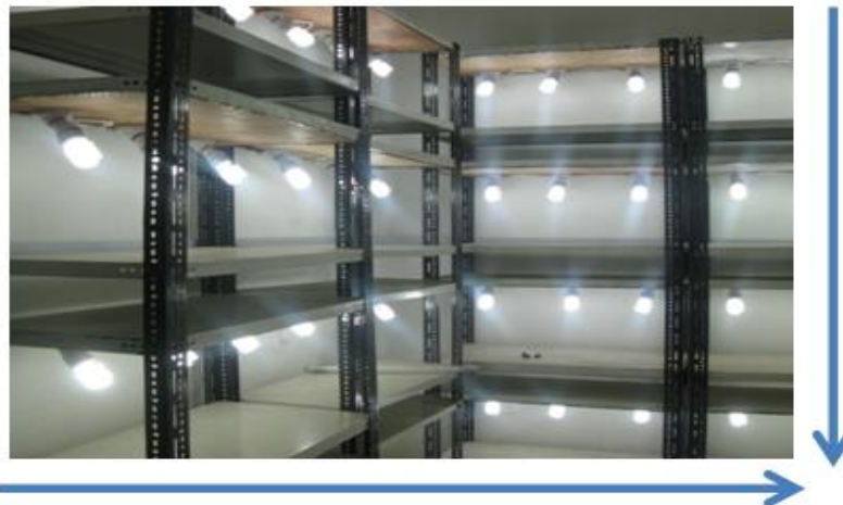
Fig.2: Serial and parallel arrangement of different intensities of plant. Showing light arranged in series across shelves (horizontal) and in parallel along racks (Vertical). Each rack is controlled by a separate switch
